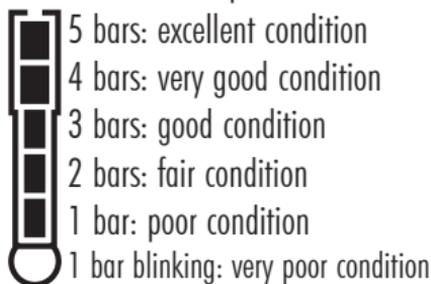
With 1 bar it is recommended to clean the electrode and recalibrate. If there is still only 1 bar or 1 bar blinking, replace the probe.
