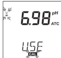
If using pH 7.01, after acceptance of the buffer press any key to exit. The “**SAVE**” message is displayed and the meter returns to pH measurement mode.
